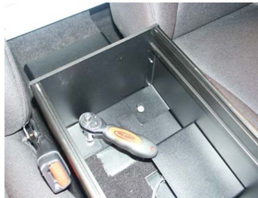
Using OEM rear bolts or 1/4" x 3/4" self threading bolts, loosely attach main console housing, sensor guard, and rear cover panel to floor (8mm or 7/16" socket)
